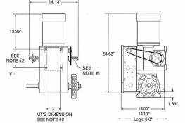
1) OUTPUT SHAFT WITH 1"x 1/4" KEY FOR 1/2 THRU 1 H.P. OPERATORS 1-3/16"x 1/4" KEY FOR 1-1/2 THRU 2 H.P. OPERATORS 1-1/4" x 1/4" KEY USED FOR 3 H.P. OPERATORS
